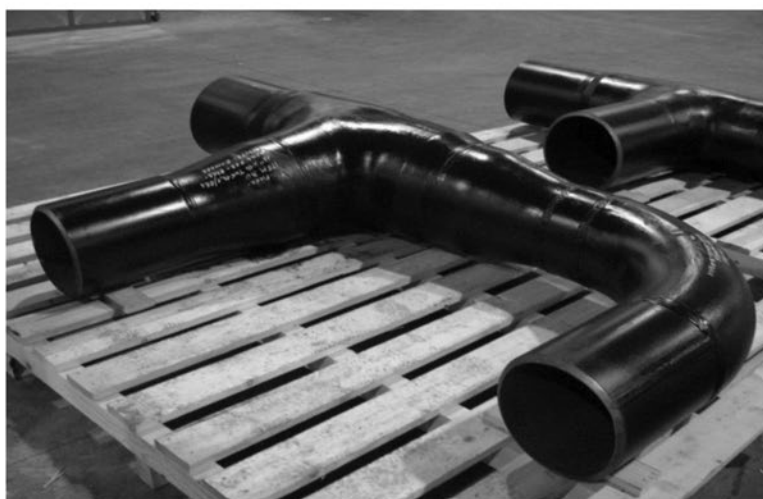
Fabricated Subsea Line-Pipe spool
