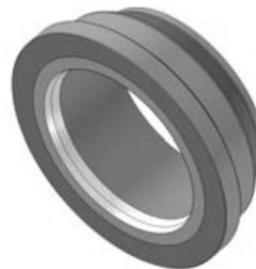
Hub weld overlaid on seal area only
