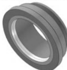
Hub weld overlaid on seal area only
